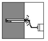
For removing the dust, clean the hole by brushes and blowing-out devices. Make sure that threaded rods or rebars are free of any contaminants, oils, greases, dust, etc.
