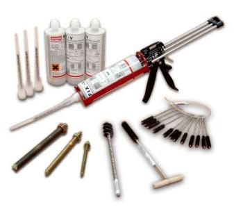
**MAXFIX®** -V is a solvent-free, vinyl ester-based resin which is packed in two-part biaxial type cartridge. It is specially designed for use by injection means. It is suitable for any solid or hollow base materials. Applications can be made easy and quick way by a chemical anchor caulking gun.
